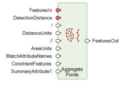
• Bridge Concavities. This operator produces an area geometry with part or all of each eligible concavity of the input area absorbed into the interior of the area by construction of a bridge that spans from one part of the boundary to another.
